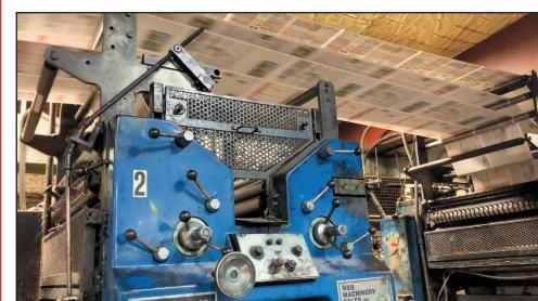
Our printer, Huron Web, takes over from here, putting our digital files onto paper thanks to a series of large, industrial "coldset" printers. This economical form of printing allows the ink to dry through evaporation and absorption into the paper. At the end of the line, the papers are folded, have their addresses labelled, and are separated into bundles to be boxed up as required for the post offices. Want to see the presses in action? Visit huronweb.net/videos
